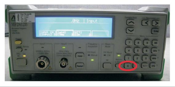
3. On the MF2412B, press the **Input** key (also the number **0** key).
