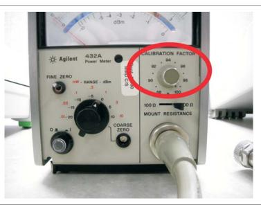
5. On the front panel of the 432A power meter, set the calibration factor to 100.
