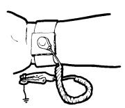
4. Wear a static-discharge wristband when working with static sensitive components.
