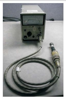
2. Connect the Agilent Power Sensor 8478B to the Agilent 432A Power Meter.
