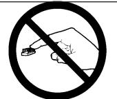
1. Do not touch exposed contacts on any static sensitive component.
