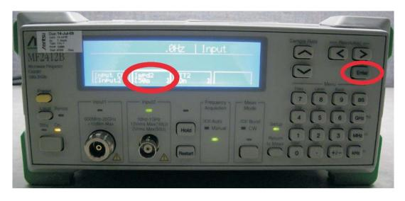
7. On the MF2412B, press the **Enter** key until **50**  $\Omega$  is selected.
