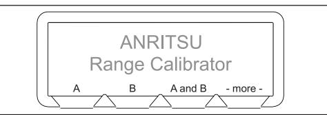
Figure 2-2. ML2419A Top Level Menu (dual-channel)
