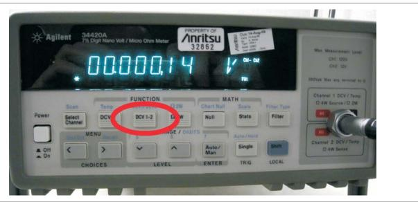
10. Select DCV 1-2 on the Agilent 34420A. Record the number shown in the display of the 34420A as  $V_o$ .
