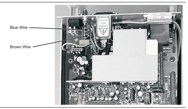
Figure 7-3. Power Supply Unit Connections
