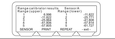
Figure 2-3. ML2419A Verification Results Menu Example
