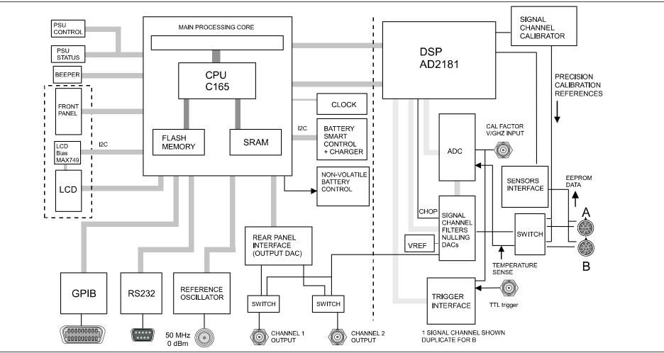
Figure 4-1. ML2430A Series Power Meter Functional Block Diagram
