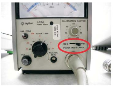
4. On the front panel of the 432A power meter, set the mount resistance to 200  $\Omega.$
