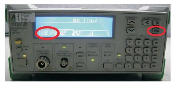
5. On the MF2412B, press the **Enter** key until **Input 2** is selected.
