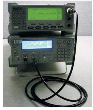
9. Connect an RF cable from **Input 2** of the MF2412B to the **Calibrator** output of the ML243xA.
