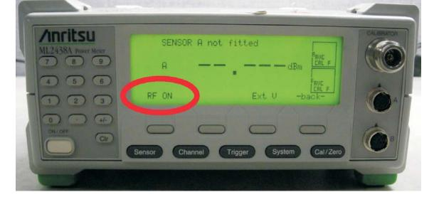
11. On the ML243xA, set the RF Calibrator to **RF ON**, by pressing the left-most soft key to change it from RF OFF to **RF ON**.
