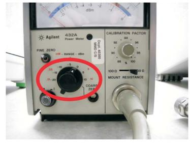
7. On the front panel of the 432A power meter, set the Range to 0 dBm.
