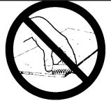
Do not handle static sensitive components in areas where the floor or work surface covering is capable of generating a static charge.
