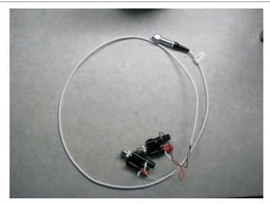
4-wire cable provided with the Agilent 34420A, along with two BNC to binding-posts adapters needed to connect the four wires to the rear of the 432A power meter.
