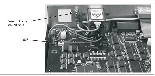
7. On the inside of the rear panel, remove the front panel ground wire (green/yellow) from the ground stud.
