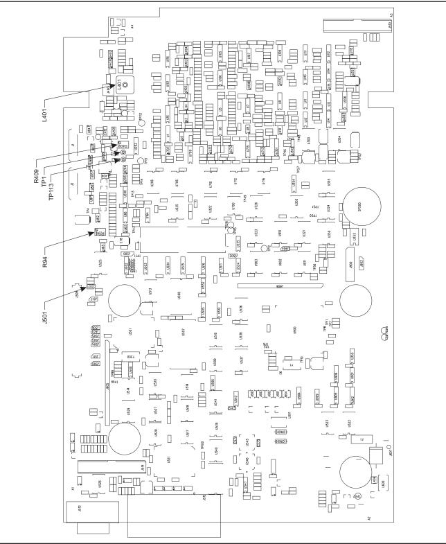
Figure 3-2. ML2430A Series Main PCB
